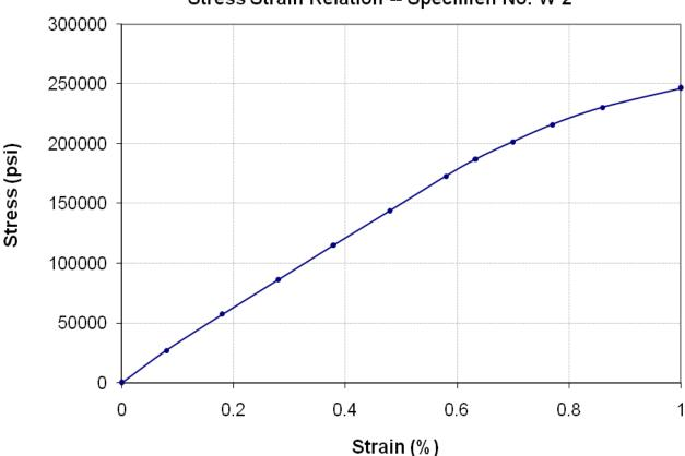
Stress Strain Relation -- Specimen No. W 2
